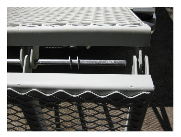
Continue to drive the rod until it is all the way through. Push the two washers against the second last set of pivot bars. Then insert the cotter pin in the hole and fold the legs of the cotter pin over. With the help of another person, lift the whole ramp up and latch each side, using the rear pocket holders. Then return the middle pocket holders back to their respective pockets. The Truck Loading Ramp installation is now complete. Now load the truck up and hit the road!
