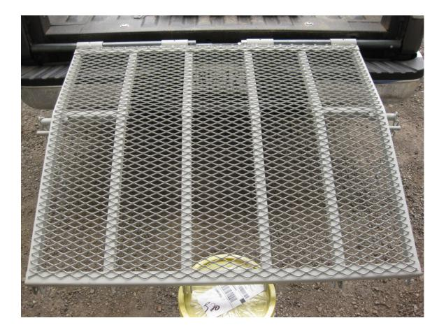
With the ramp properly supported insure that the ends of the shaft are touching the sidewall of the tailgate opening. After confirming this, lock the shaft in place. To do this run the nylon insert nut, which is provided and mounted on the threaded rod, until it is against the left side shaft.
