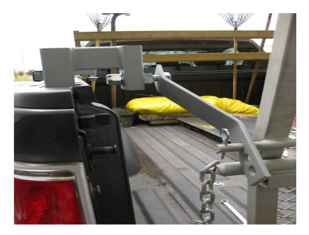
With the rear pocket assemblies completed, drop them into the rear pockets of the truck. Then (with the help of another person) lift the curved ramp half up and using the latch on the rear pocket holder, secure the gate in place. **Do not forget to put on the hitch pins.**
