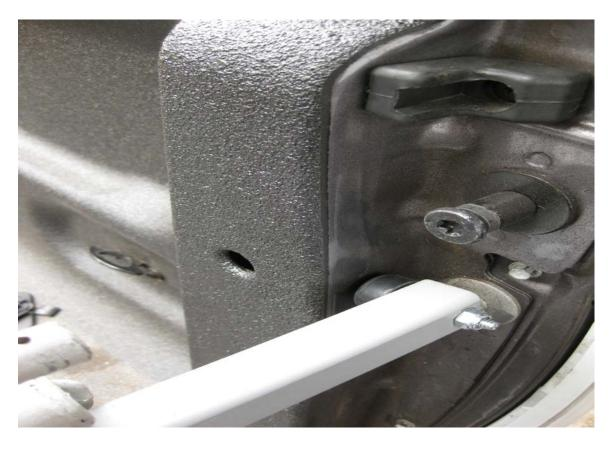
Maintain the position of the stopper tubes and drill a  $^{1}/_{4}$ " hole through the tube. Refer to the picture below.
