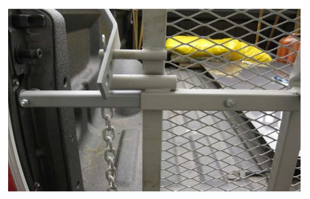
With the stoppers is in place, assemble the middle pocket holders. The middle pockets are directional, so it is best to place the pocket holders into the pockets of the truck, and the follow the steps listed.
