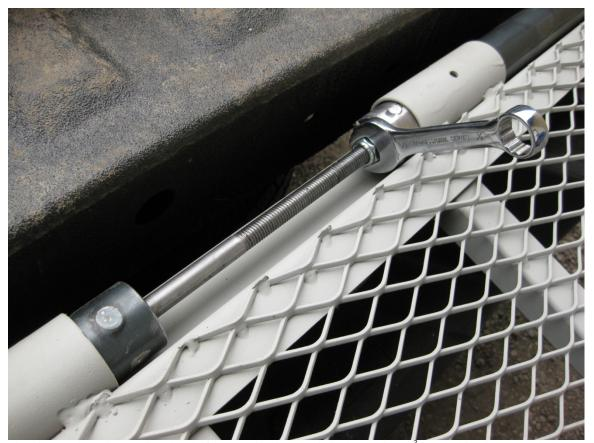
The Picture above is showing the shaft locked in place. This is done using a <sup>3</sup>/<sub>4</sub>" combination wrench.
