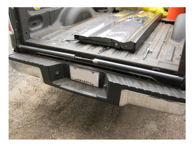
Now that the proper length has been finalized, slide the shaft through the first half of the Truck Loading Ramp (curved half). Place both the shaft and ramp back on the tailgate pivots with something to support the ramp underneath. The picture on the next page shows the ramp being supported by a 5 gallon pale. This pale should preferably be **filled**, as this will be helpful later in the process.
