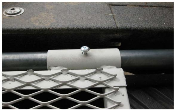
Now that the two end holes have been drilled and bolted, the rear pocket assemblies must be put together. But first, remove the caps for the pockets using a flat head screw driver. See the reference picture below.
