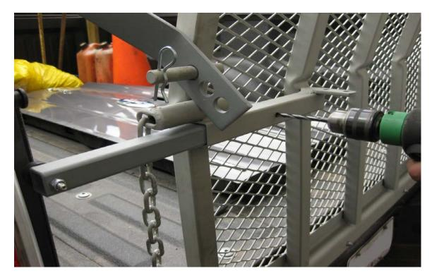
Then using  $\frac{1}{4}$  x  $1^{3}/4$  bolt, secure the stopper tube. Refer to the picture below.
