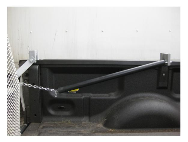
The final assembly of the spring connection, from ramp to middle pocket holder, should look like the picture above.
